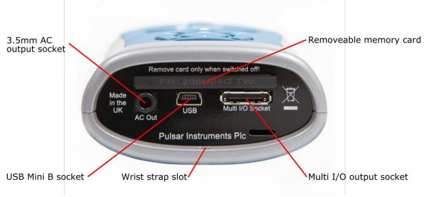
The Nova® can be powered via the multi-pin connector on the bottom of the instrument.
