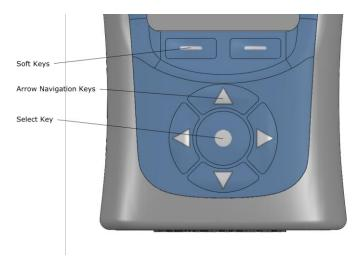
The ambient light sensor on the front of the instrument will illuminate the elastomer keypad and adjust the brightness of the display automatically when the light level falls.
