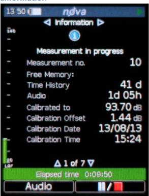
This shows the status of the instrument including the calibration data.
