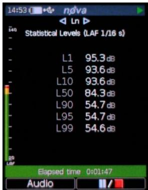
The Ln view shows the statistical or Ln values calculated during the measurement.
