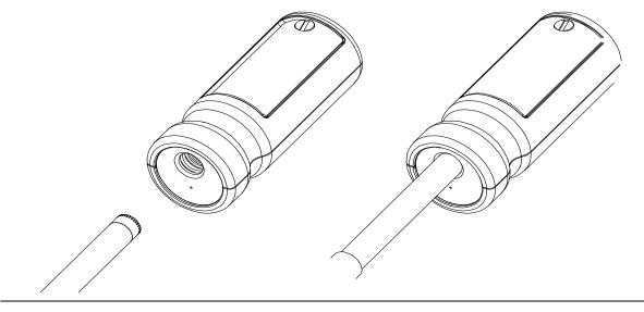
The Nova® sound level meter will automatically make adjustments for the level produced by the acoustic calibrator and the microphone type fitted to the instrument.
