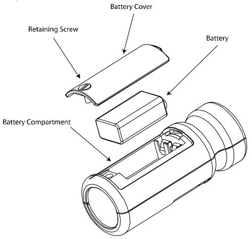
2. The battery, type 6F22 (PP3) can now be eased out of its holder and replaced. The battery should be eased out terminal side first by pushing against the spring at the other end.
